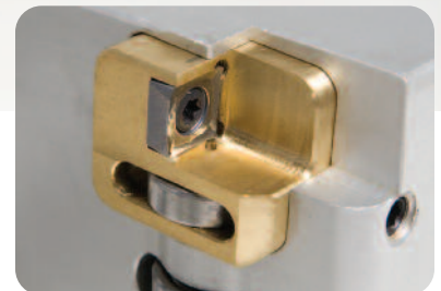
Spring loaded, floating blade carriage handles uneven pipe surfaces with ease. Four sided, field replaceable blade is easy to rotate to a new cutting surface.
